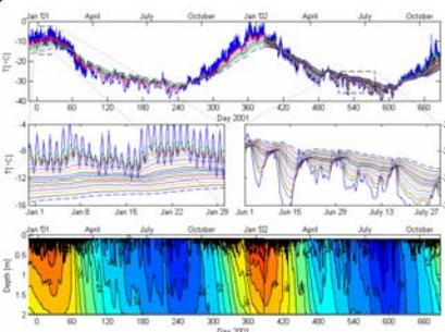
Figure 2. Temperature data and reconstructed temperature field at site TM2. Top plots show  $T(t)$  traces for each thermistor. The bottom thermistor ( $z = 1.98$  m) is the dashed line, top thermistor ( $z = 0.09$  m, in surface debris) has the largest amplitude. Only every second thermistor is shown in the top figure.
