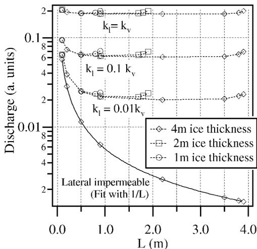
Fig. 4. Relationship between discharge and ice thickness  $L$  underneath the borehole in a simulated bail-test geometry. The model runs are performed in ice with  $k_l/k_v = 1$  (isotropic), 0.1, 0.01 and 0 (laterally impermeable). The hydraulic head is kept constant. The total ice thickness is 1, 2 and 4 m.
