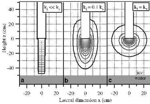
Fig. 3. Model calculations of the pressure field during a bail test for three different ratios between lateral permeability  $k_l$  and vertical permeability  $k_v$ . In a vertical cross-section the initial isobars are plotted for constant intervals. (a) The simulation with laterally impermeable ice; (b) the case for a ratio of  $k_l/k_v = 0.1$ ; and (c) the isotropic case with  $k_l = k_v$ .
