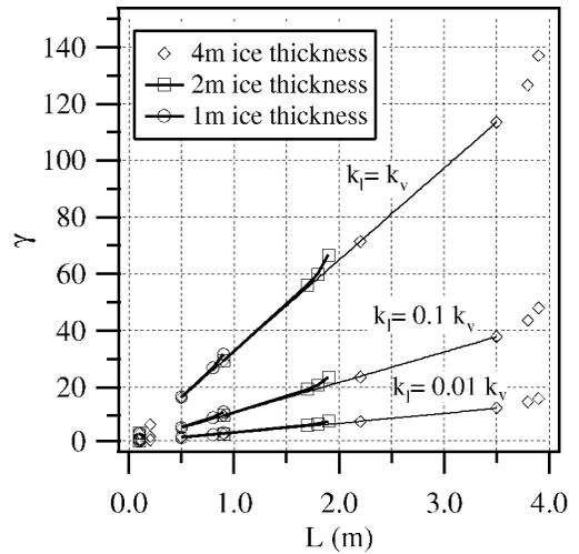
Fig. 5. Relationship between the derived correction factor  $\gamma$  and ice thickness  $L$  underneath the borehole.  $\gamma$  depends linearly on  $L$  with rising slopes for increasing  $k_l/k_v$  ratio which reflects the enhanced inflow due to lateral permeability.
