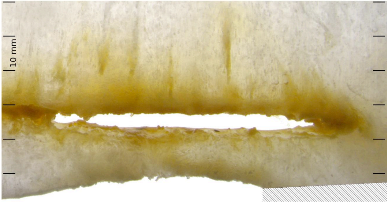
Figure 2. Vertical section of (synthetic) oil-infiltrated ice surrounding an overgrown oil lens in an experiment equivalent to Exp 20. Gradation at the sides is in 10 mm.
